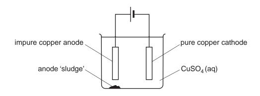
The impure copper anode contains small quantities of metallic nickel, zinc and silver, together with inert oxides and carbon resulting from the initial reduction of the copper ore with coke. The copper goes into solution at the anode, but the silver remains as the metal and falls to the bottom as part of the anode 'sludge'. The zinc also dissolves.
