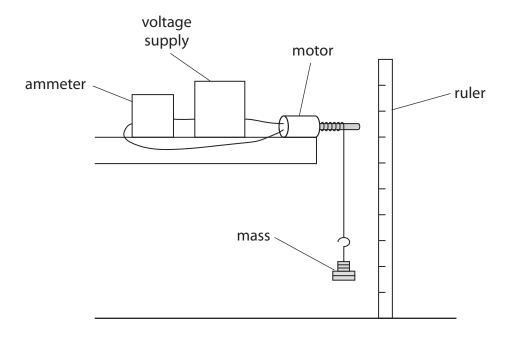
The current in the motor is 2.1 A and the voltage across it is 12 V.
